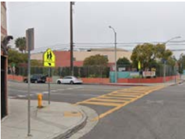
A ladder crosswalk with pedestrian crossing signage, East Los Angeles.
